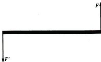
Figure 4-27. A pair of parallel forces of equal magnitude acting in opposite directions but not on the same point is called a couple. (The weight of the bar is not considered in this example.)
